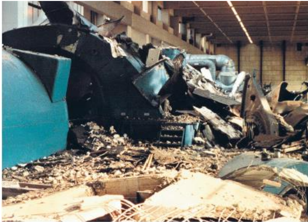
This overall view of a generator shows the damage done to the inboard end during a steam turbine overspeed event. Notice the absence of coupling and turning gear that were ejected.
