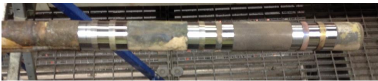
Long-term clamp exposures - convective HXs and Intrex tubes -
