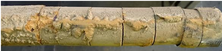
Short- and long-term fouling probes - backpass conditions -
