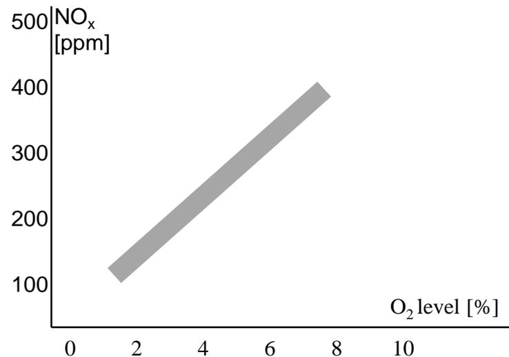
*Optimization of terminal oxygen level on the grounds of CO-emission rate reduces NO<sub>x</sub>–emissions. Stabilization of combustion power and air controls enables the boiler's running at lower terminal oxygen content than earlier.*
