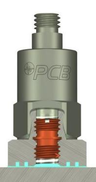
To generate a useful output signal, the sensors rely on the piezoelectric effect. ("Piezo" is a greek term which means "to squeeze.") When the piezoelectric elements are strained by an external force, displaced electrical charge accumulates on opposing surfaces.
