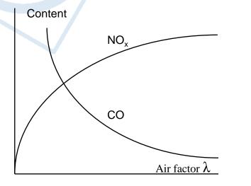
Optimization of terminal oxygen level on the grounds of CO-emission rate reduces  $NO_x$  – emissions. Stabilization of combustion power and air controls enables the boiler's running at lower terminal oxygen content than earlier.
